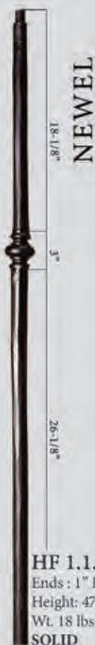
HF 1.1.22 Ends: 1" Rd. Height: 47-1/4" Wt. 18 lbs. SOLID
