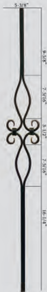
HF 16.8.9 Ends : 5/8" Sq. Height: 44" Wt. 4 lbs. TUBULAR
